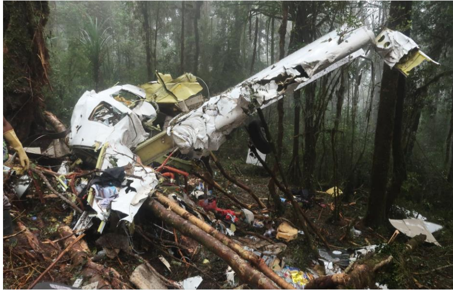
Figure 14: The fuselage and left wing condition
