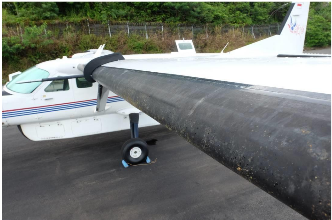
Figure 11: The wood impact marks on left wing
