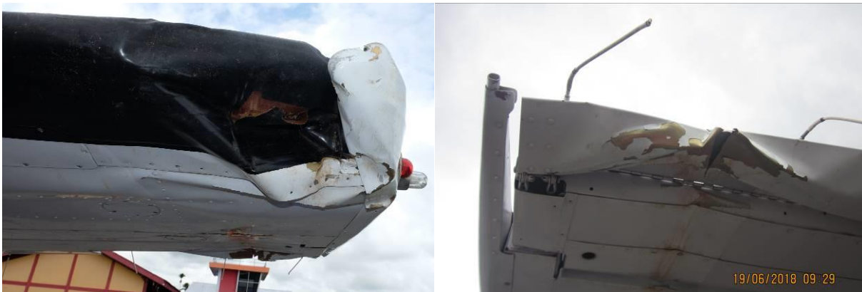
Figure 2: The damage on the left wing tip
