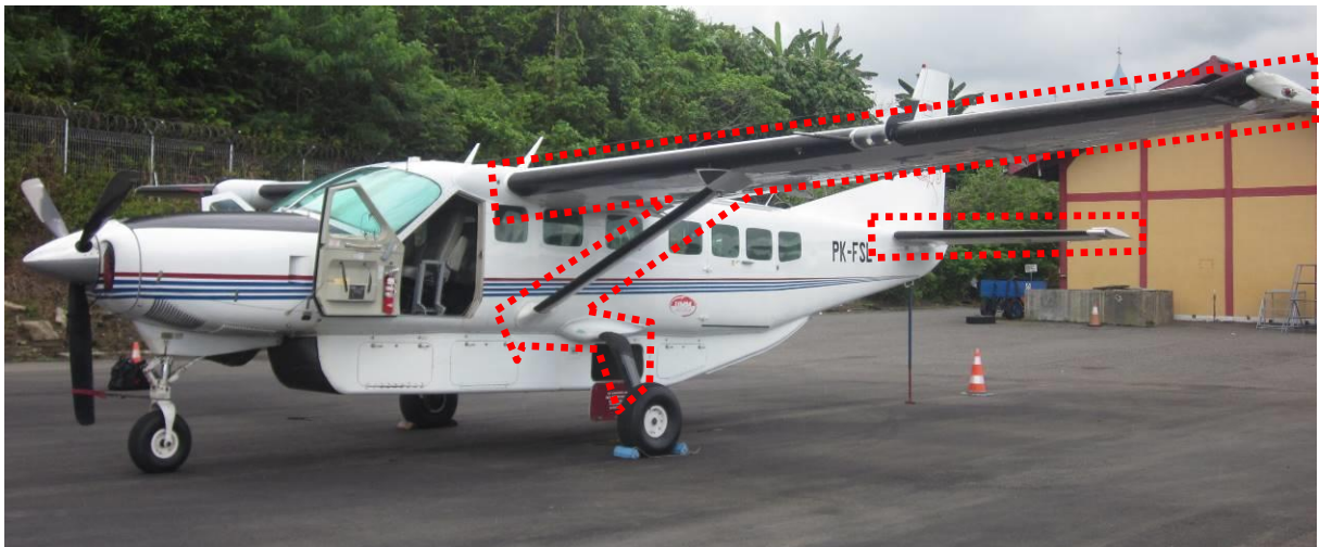
Figure 9: The impact marks on the aircraft (inside the red dot line)
