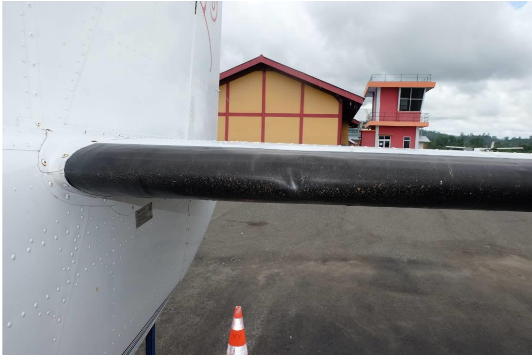
Figure 12: The dent and impact marks on left horizontal stabilizer
