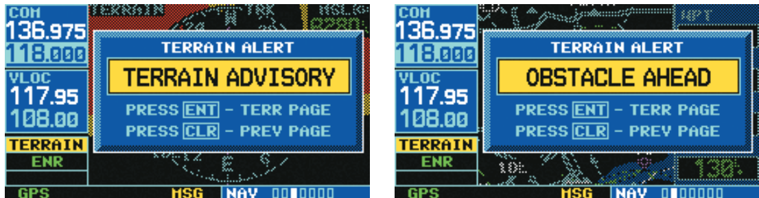
Figure 6: The advisory pop-up (left) and flashing caution pop-up (right)
