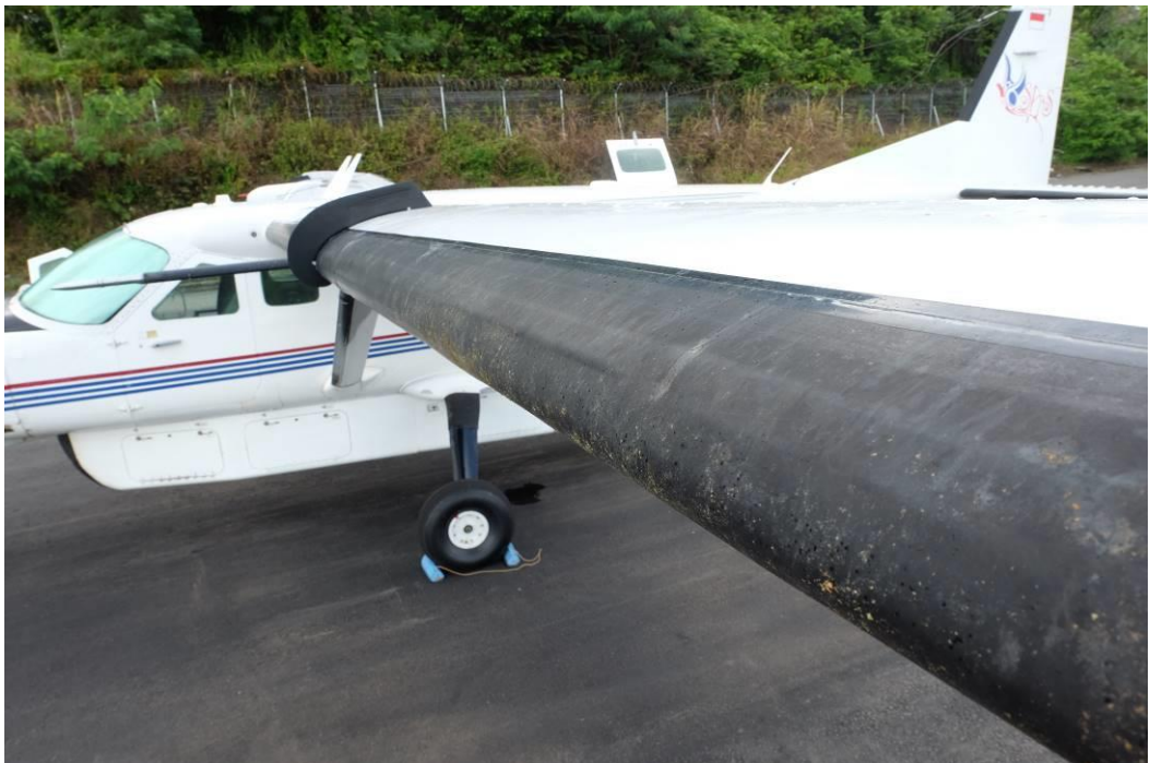
Figure 15: The wood impact marks on left wing leading edge
