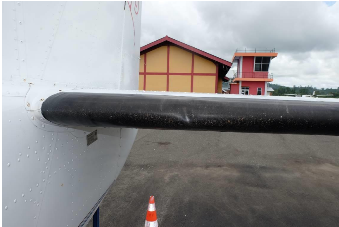
Figure 16: The dent and impact marks on left horizontal stabilizer
