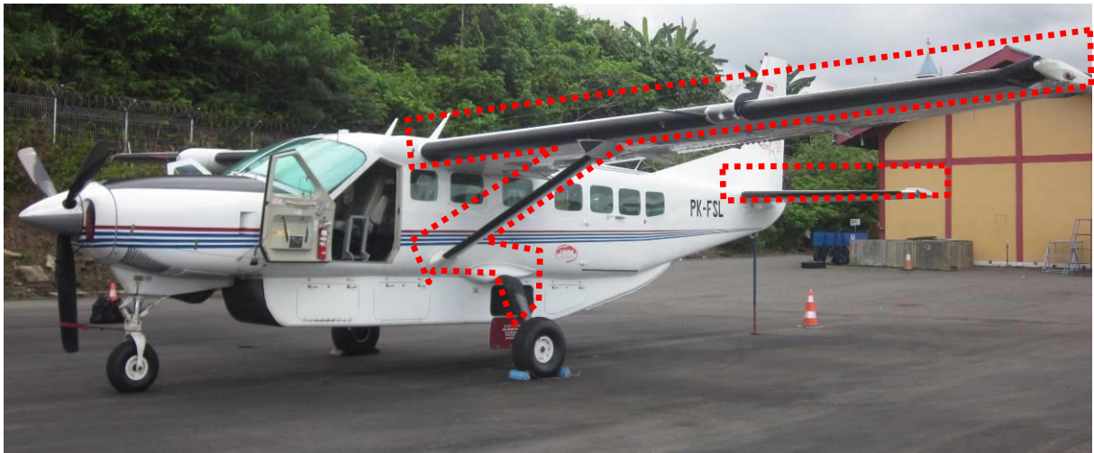
Figure 13: The impact marks on the aircraft found in the area inside red dot lines
