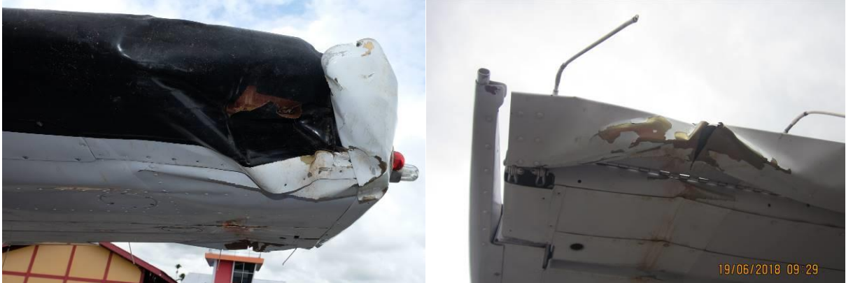
Figure 2: The damage on the left-wing tip and left aileron
