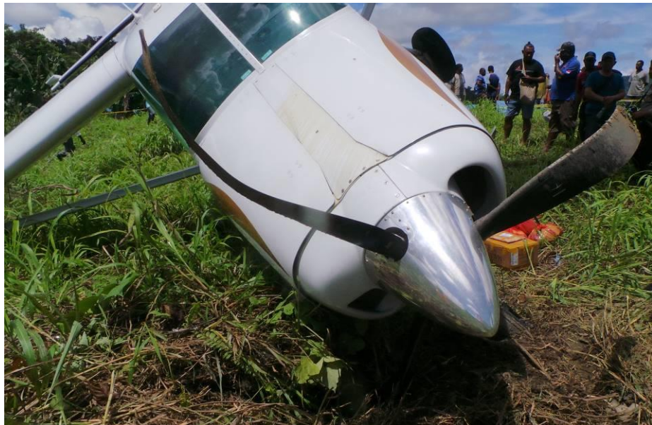
Figure 3: The propeller bent backward
