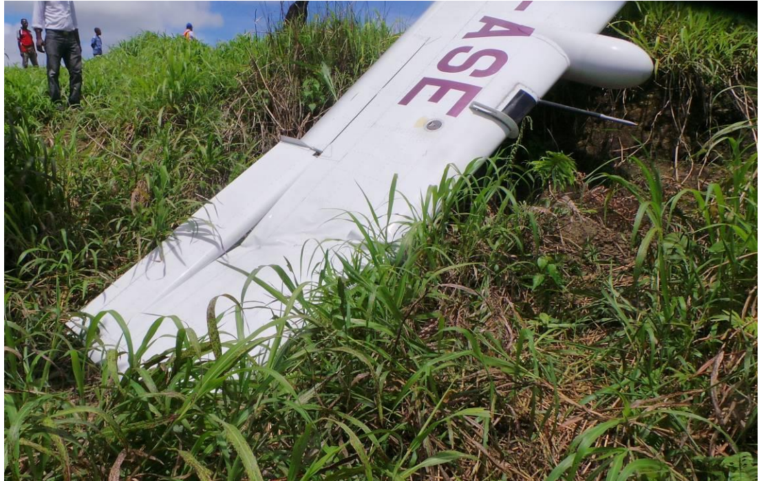
Figure 4: The damaged right wing
