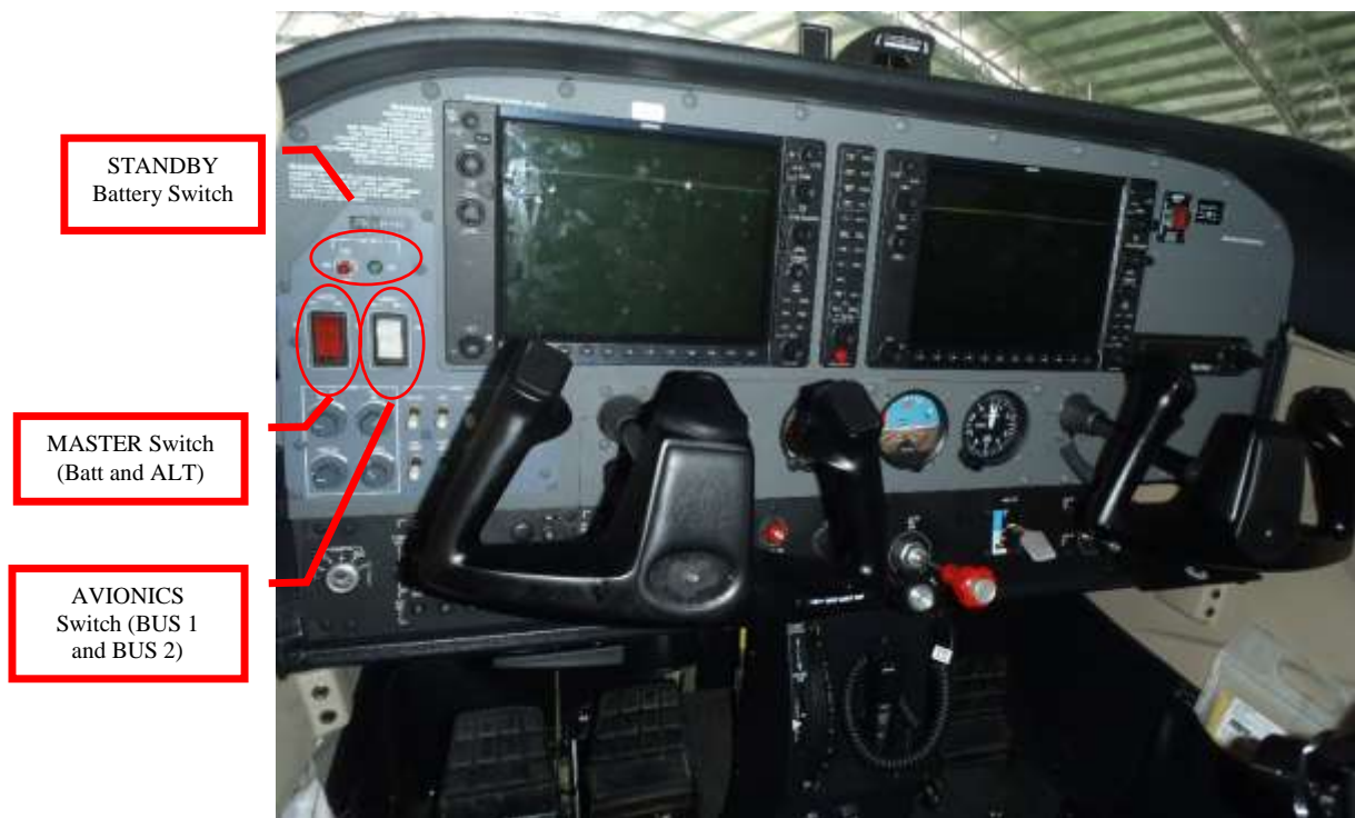
Figure 5: The electrical system switch position
