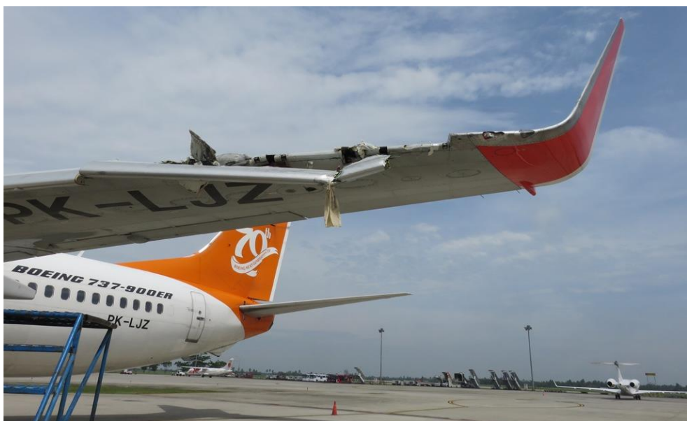
Figure 7: The damaged wing of JT197
