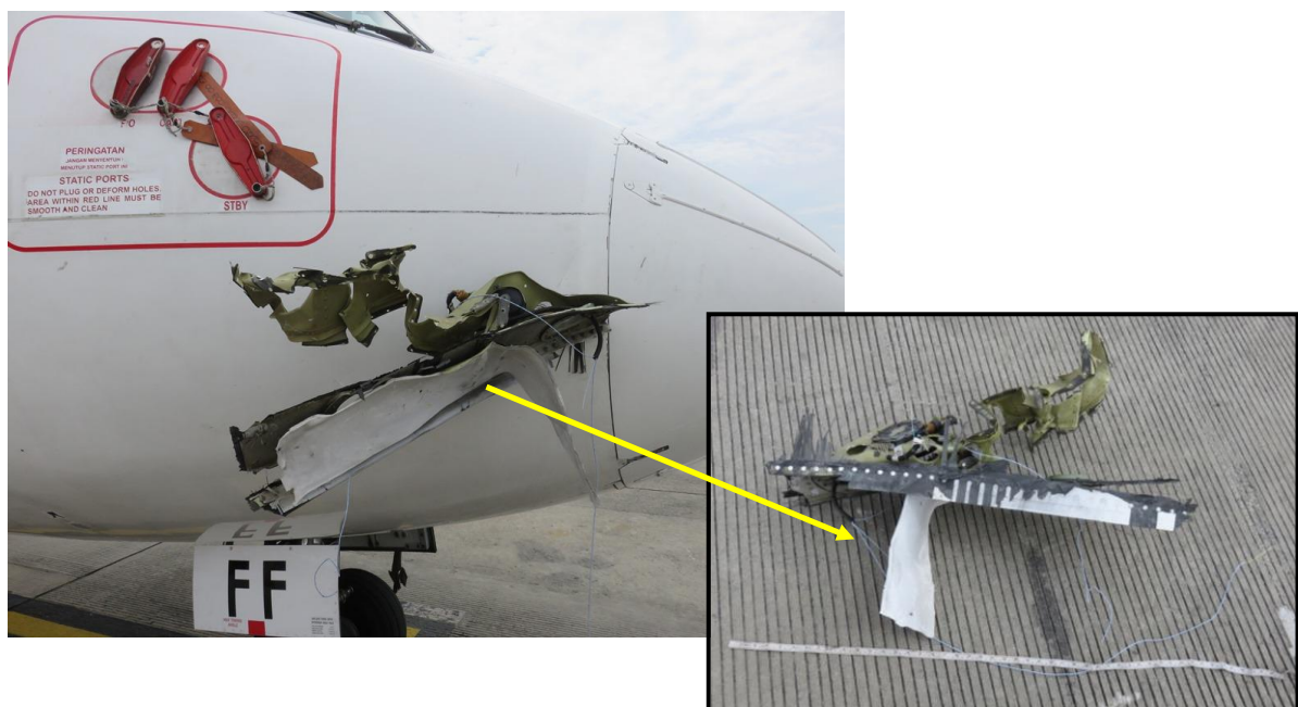
Figure 13: Part of the damaged wing that stuck at the pitot tube
