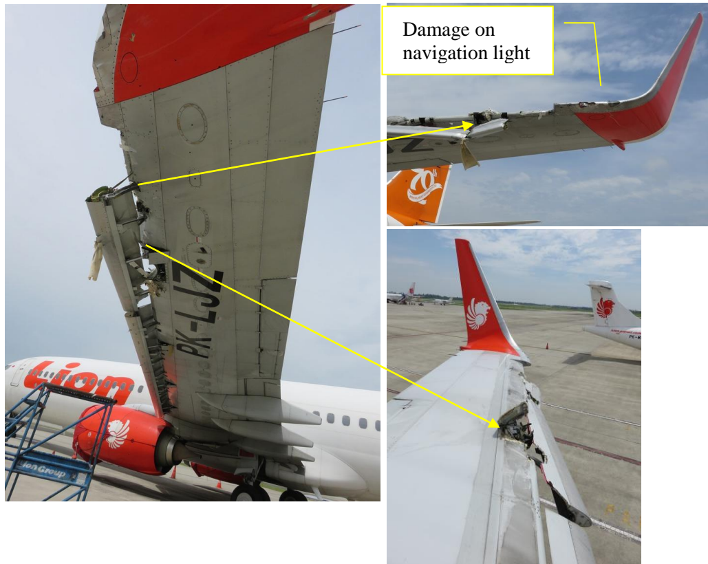
Figure 8: The damage on the left wing of JT197
