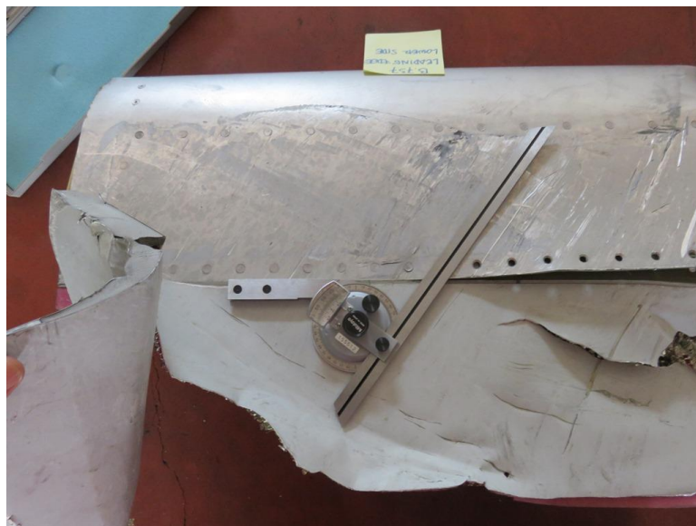
Figure 9: Part of slat number 1 recovered from the runway
