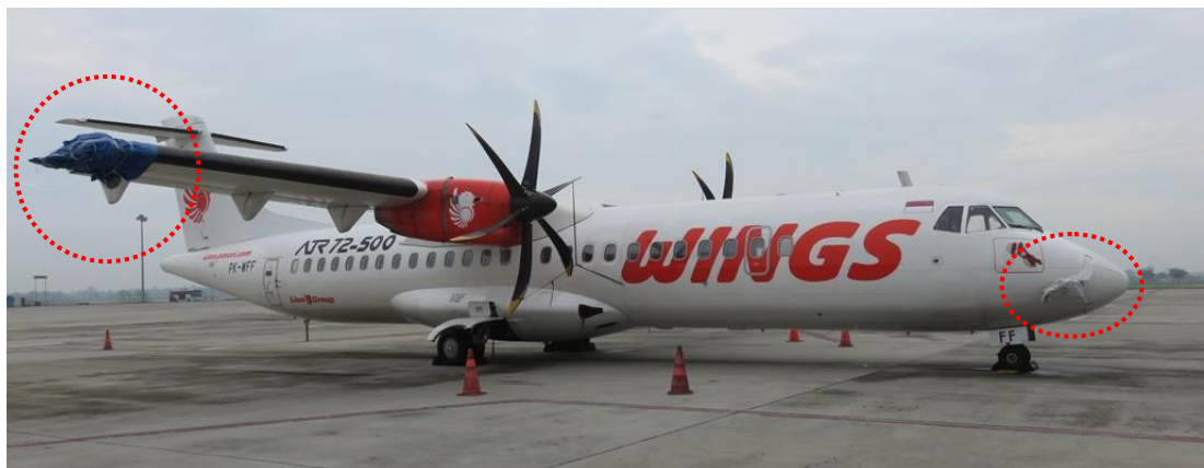
Figure 11: Damage on the right wing with part of the wing striking the pitot tube
