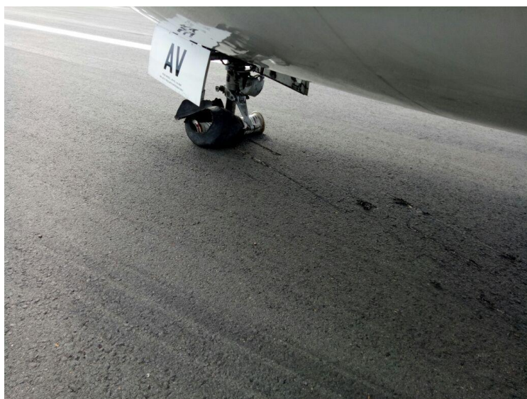
Figure 2: nose landing gear damaged
