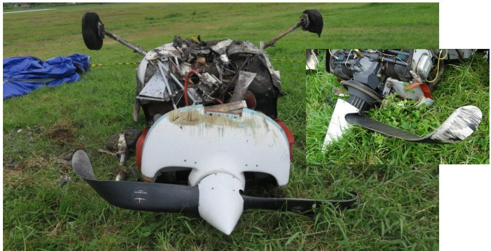
Figure 3: The propeller, engine and engine cowling condition after the accident
