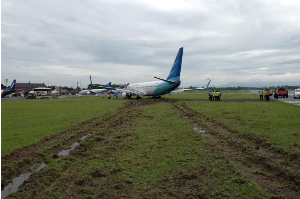
Figure 1: The wheel marks on the shoulder and aircraft condition after stopped
