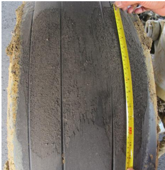
Figure 11: Reverted rubber mark on main wheel
