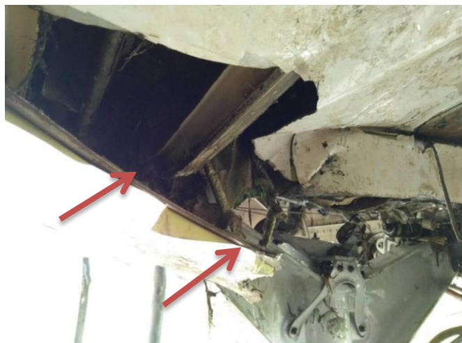
Figure 1: Damage on the lower frame bulkhead of the nose landing gear compartment
