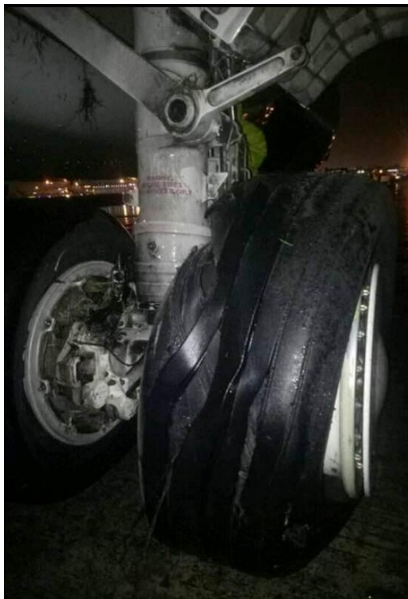
Figure 7: The burst outer tire of right main landing gear
