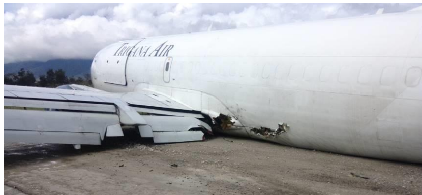
Figure 3: Damage on the lower fuselage
