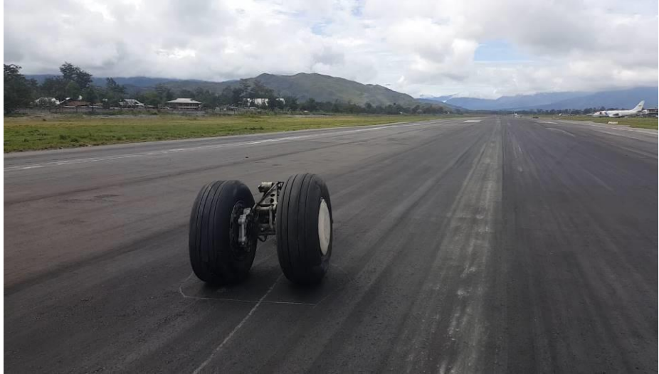
Figure 10: The left main landing gear found on the left side of the white paint scratch mark
