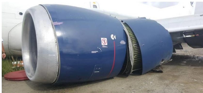
Figure 4: Damage on the left engine
