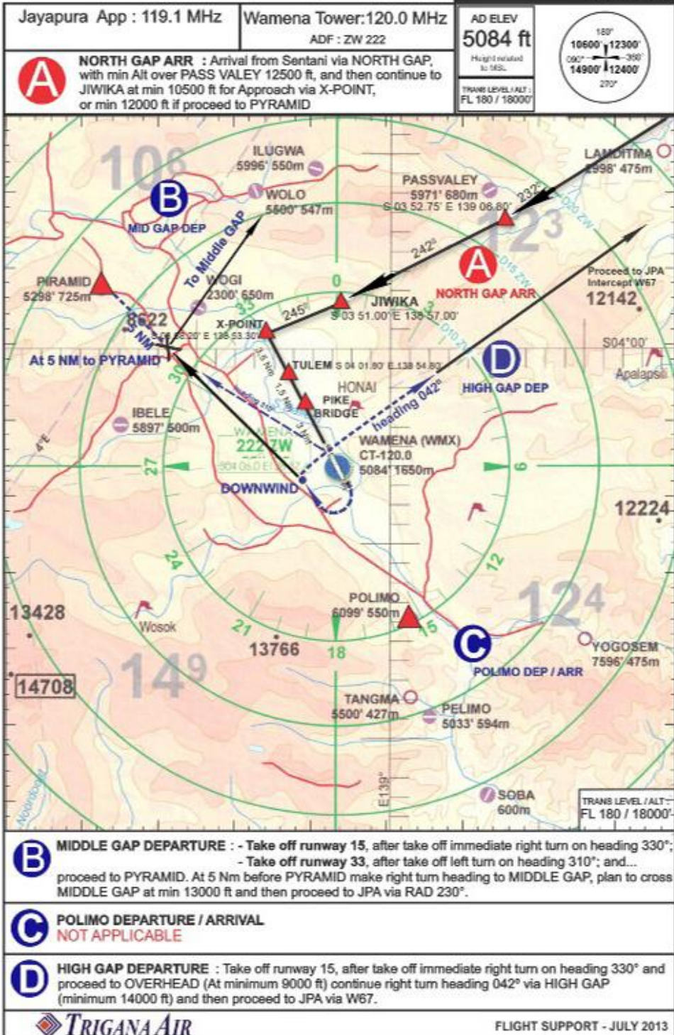
Figure 6: Operator Visual Guidance, terminal area chart
