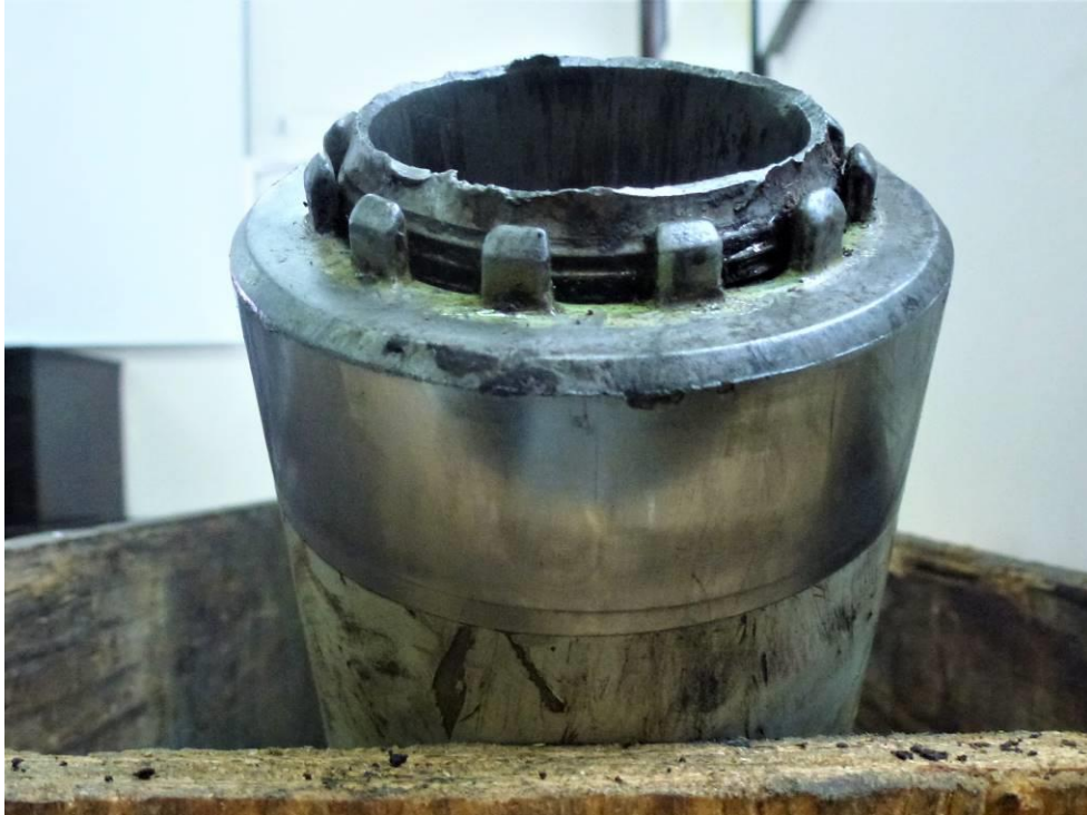
Figure 13: the broken surface of the left main landing gear strut
