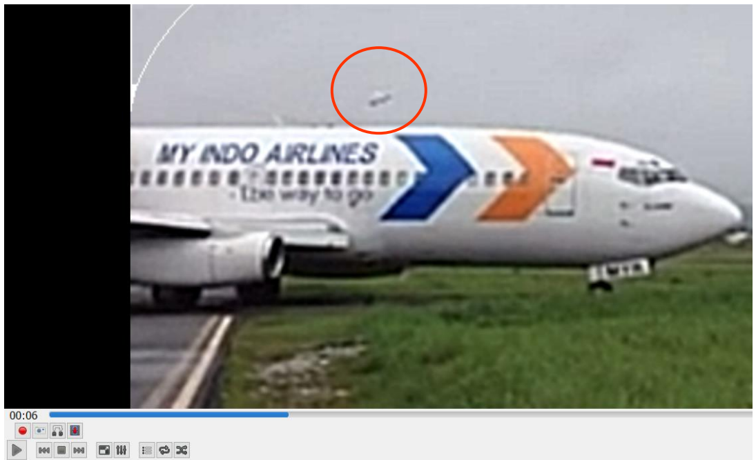
Figure 16: At video time 00:06, the aircraft was rolling to the right and pitching down
