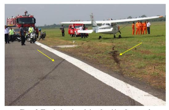
Figure 3: The wheel marks and aircraft position after stopped
