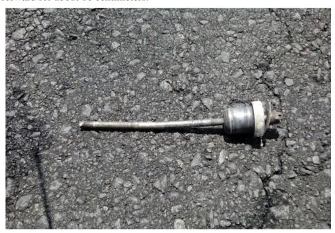
Figure 2: the nose wheel axle through bolt found on runway
