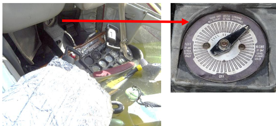
Figure 6: The fuel selector valve position found after impact
