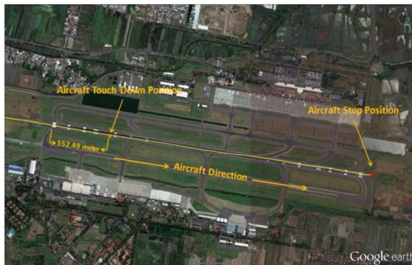
Figure 5: The landing trajectory processed from the FDR
