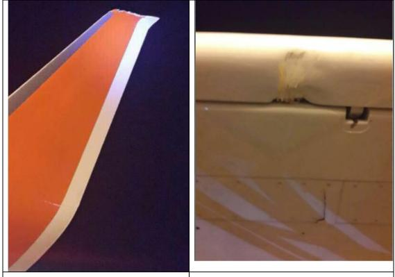
Figure 2: LNI770 left winglet cut off
