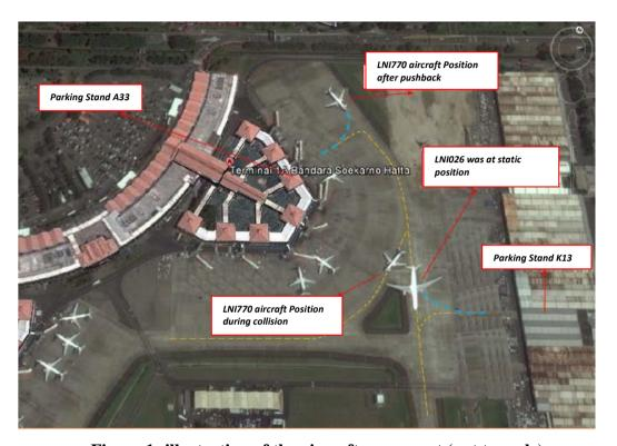
Figure 1: illustration of the aircraft movement (not to scale)
