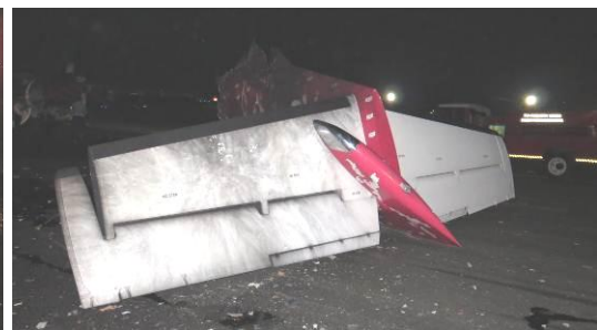
Figure 5: The detached parts of wing and horizontal stabilizer
