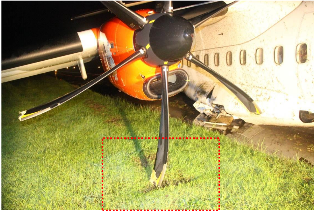
Figure 13: The propellers condition and scratch mark on the ground
