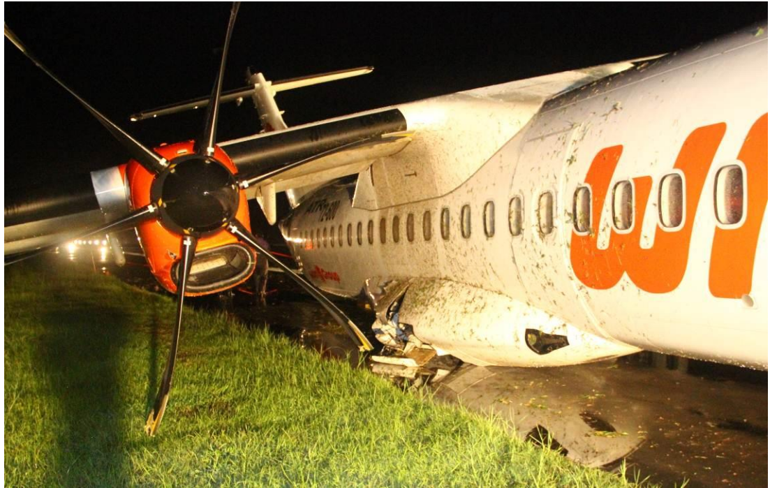
Figure 2: The damaged main landing gear and propeller
