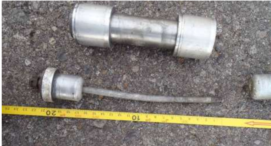
Figure 2: the nose wheel axle components (castellated nut, washer and cotter pin) found on runway separately
