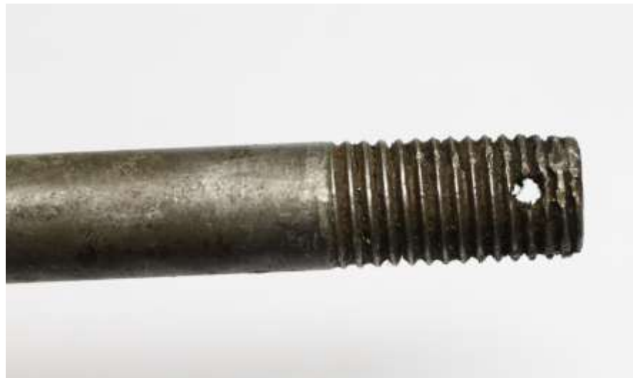
Figure 8: The dirt in the hole of the axle stud
