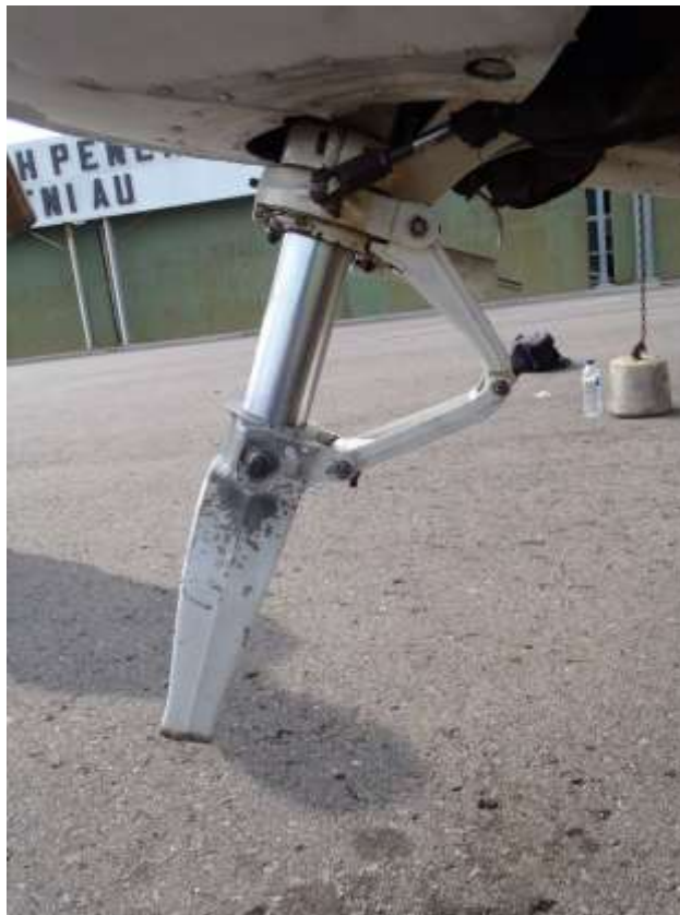
Figure 3: The scrap on nose wheel fork
