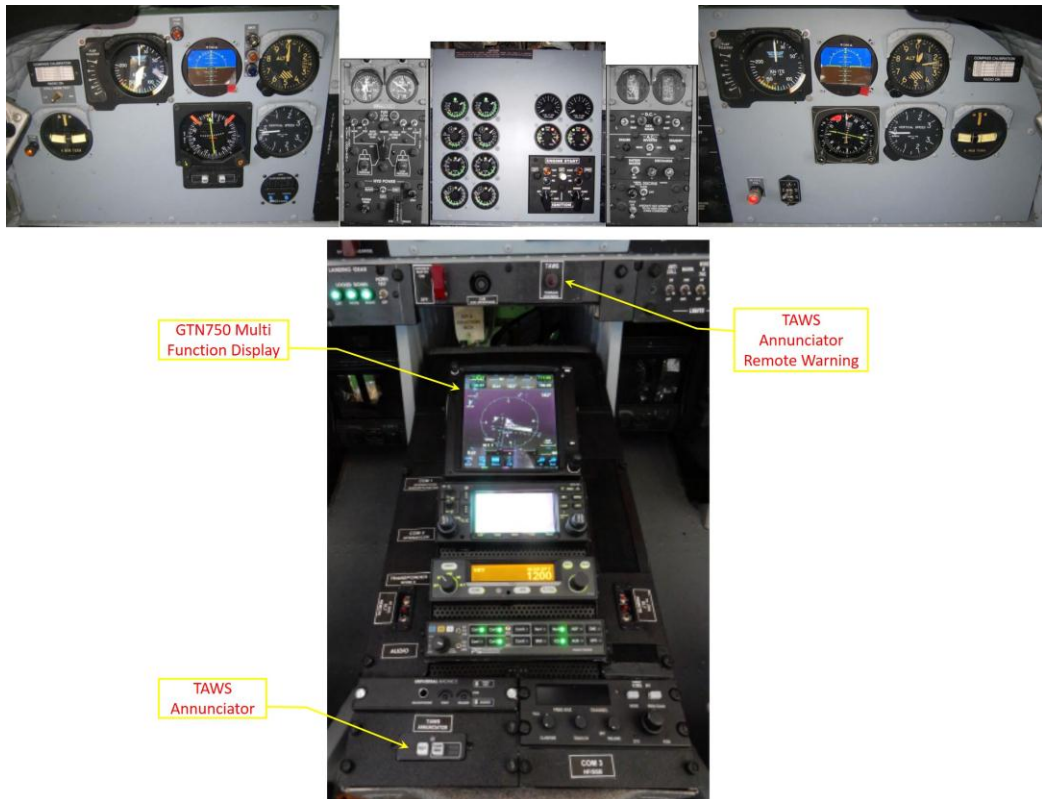
Figure 3: The cockpit layout after modification
