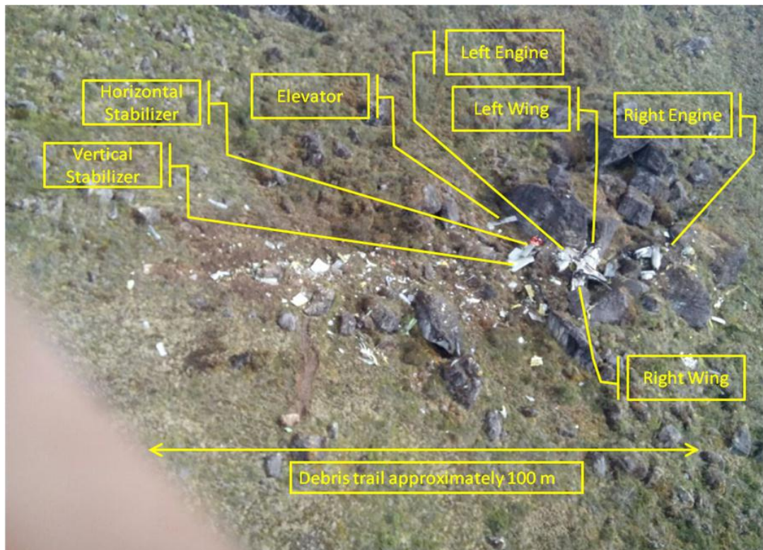
Figure 11: The wreckage distribution
