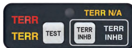
Figure 5: The MD41-1208 annunciator light and terrain control
