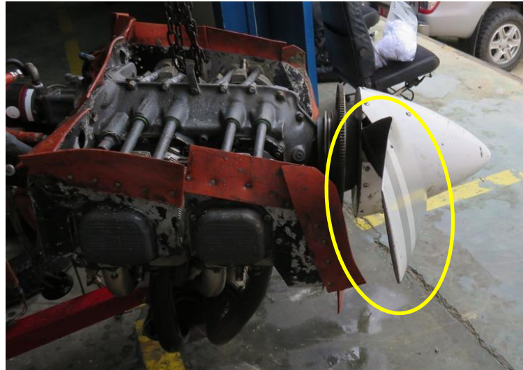
Figure 12: The bend to the propeller blade
