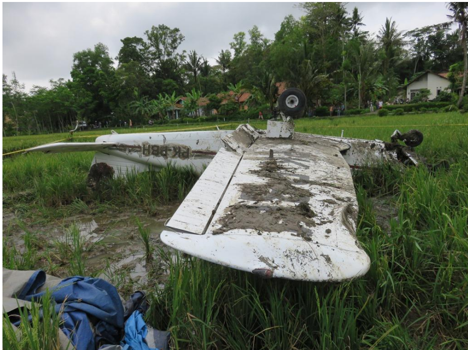
Figure 2: The damage on the left wing
