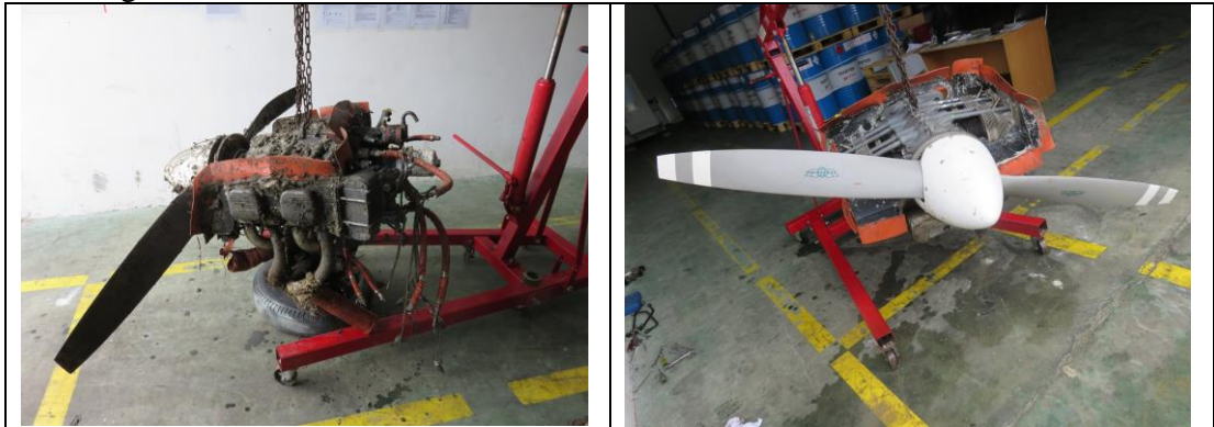
Figure 11: The engine before and after washed
