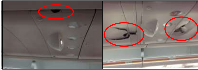
Figure 11: Damage on passenger service units
