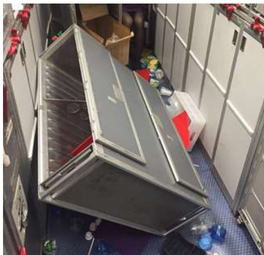
Figure 10: The aft galley condition after encounter turbulence
