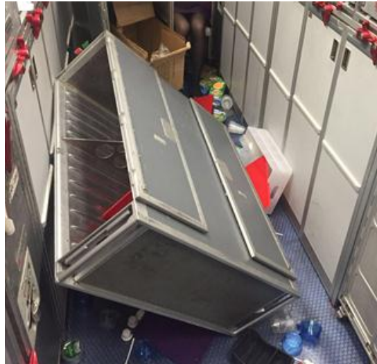
Figure 9: The aft galley condition a few minute after turbulence
