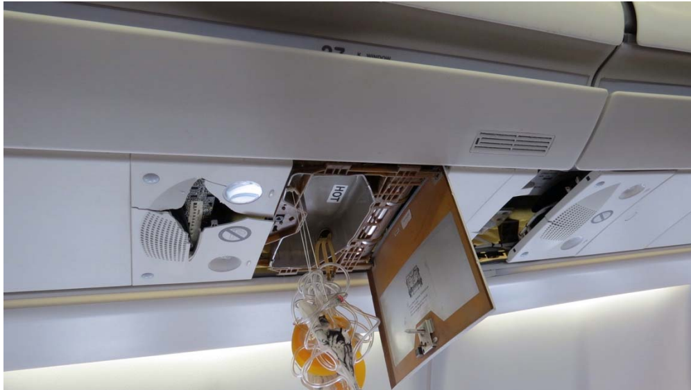
Figure 4: The damaged passenger service unit
