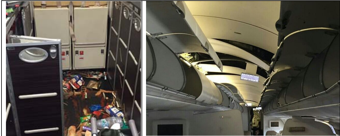
Figure 2: Aft Cabin ceiling and mid galley condition after the severe turbulence
