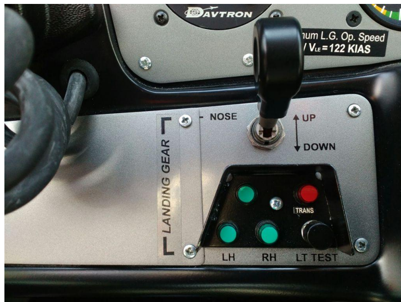
Figure 4: The landing gear handle found at UP position
