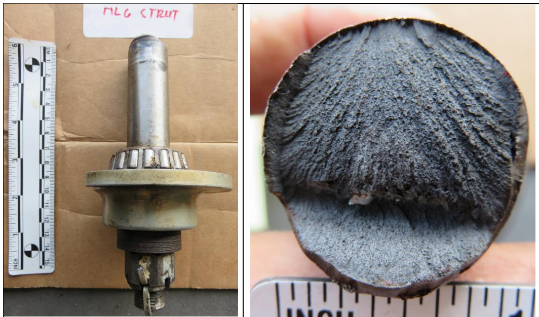
Figure 3: The collapsed nose landing gear strut (left) and its collapsed surface (right)
