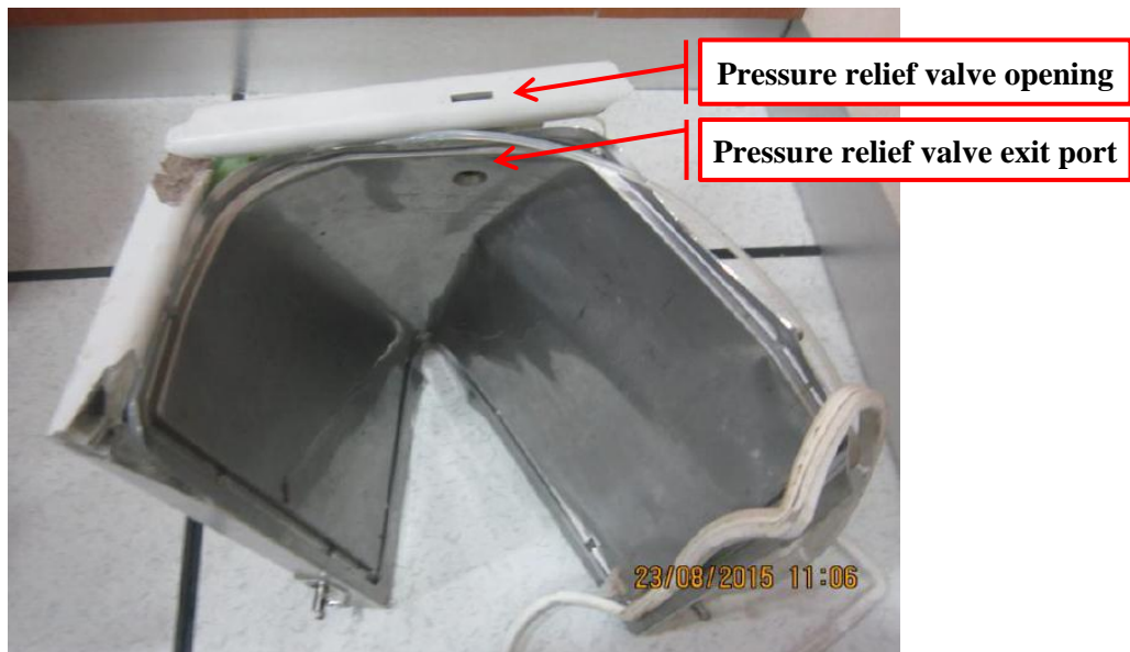
Figure 8: The deformation of the separated door (note: the time stamp was the camera time and was not set correctly)
