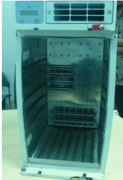
Figure 7: Bulging on the refrigeration unit
