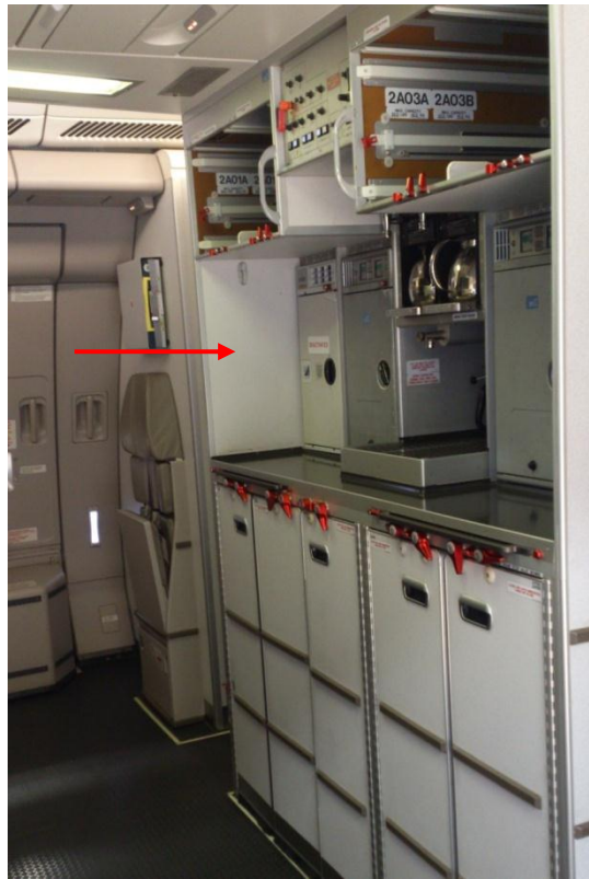
Figure 6: The location of the refrigeration unit in middle galley
