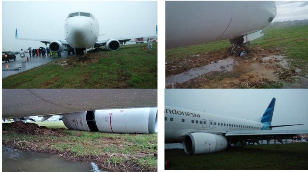
Figure 3: Aircraft position and condition after stop
