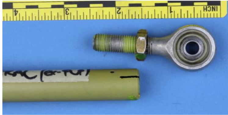
Figure 42: Rod end bearing was unscrewed from the push rod assembly
