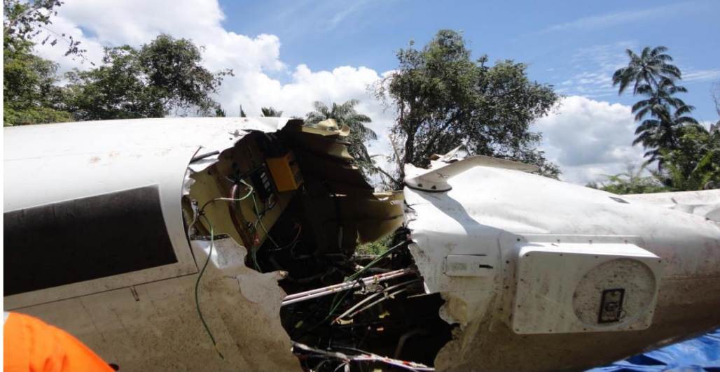
Figure 15: Broken tail boom
