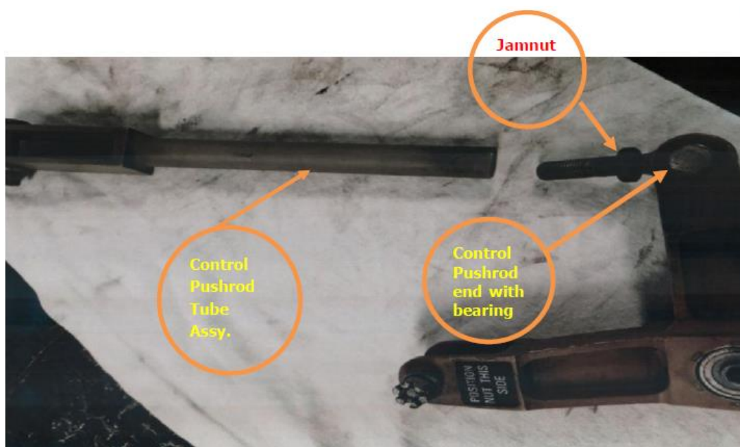
Figure 50: The rod end bearing was separated from the push rod
