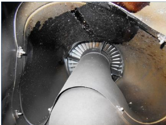
Figure 25: Left engine exhaust condition
