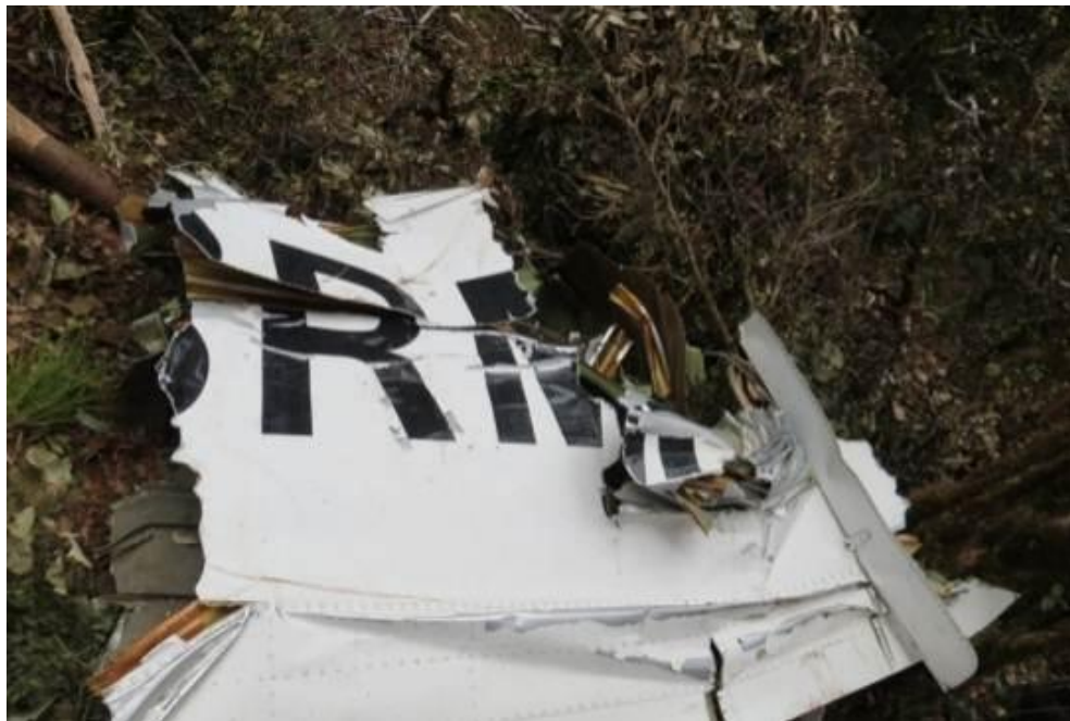
Figure 5: Part of the right wing found approximately 100 meters from the main wreckage
