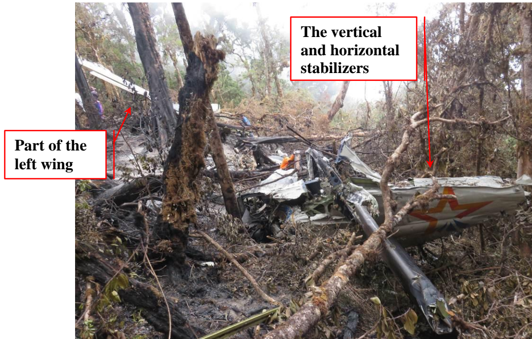
Figure 6: Main wreckage and the distribution of aircraft part
