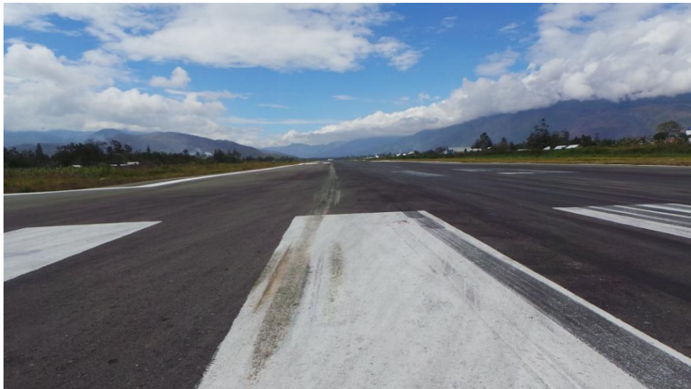
Figure 9: Metal scratch mark started from the runway threshold until aircraft final position
