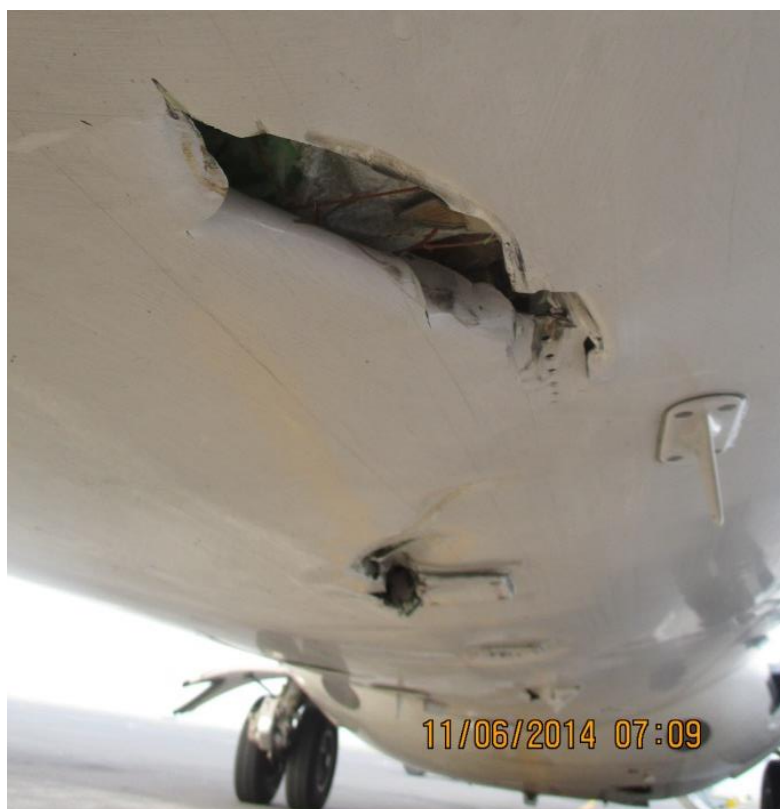
Figure 3: Damages found on the lower fuselage
