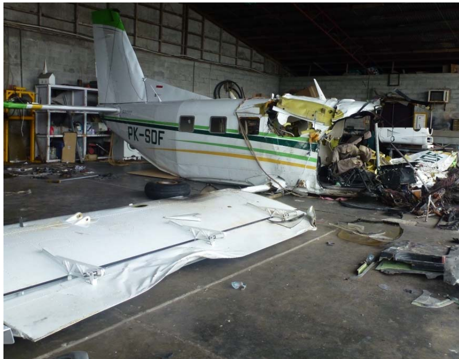
Figure 8: Wing flap physically did not extend
