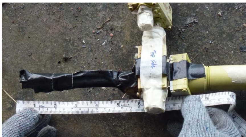
Figure 10: Measurement of the wing flap screw jack
