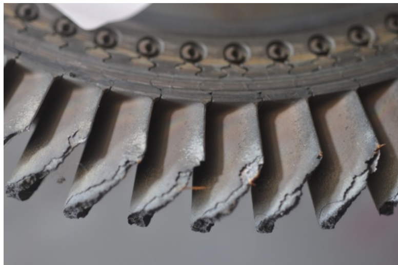
Figure 14: Broken blades of the compressor turbine
