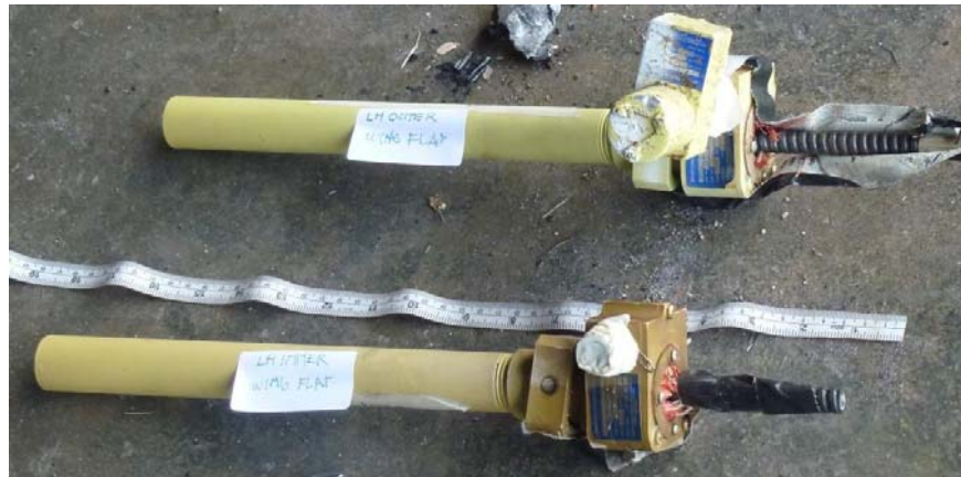
Figure 9: The left inner and outer wing flap screw jacks
