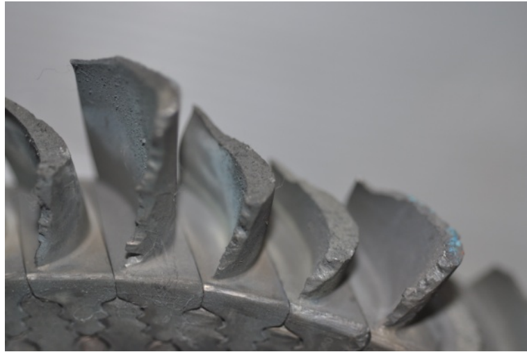
Figure 15: Broken and deformed PT blades
