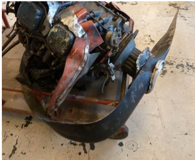
Figure 7: The propeller blade bent backward
