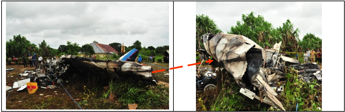
Figure 10: The deformation of the left wing leading edge
