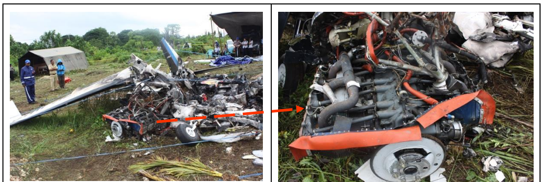
Figure 14: Right engine condition
