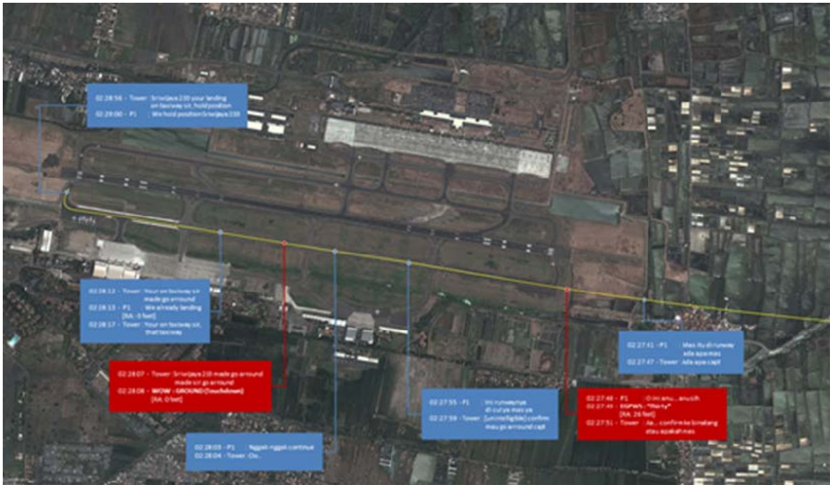
Figure 5: The aircraft flight and on SP2 taxiway trajectory revealed from the FDR plotted to Google earth
