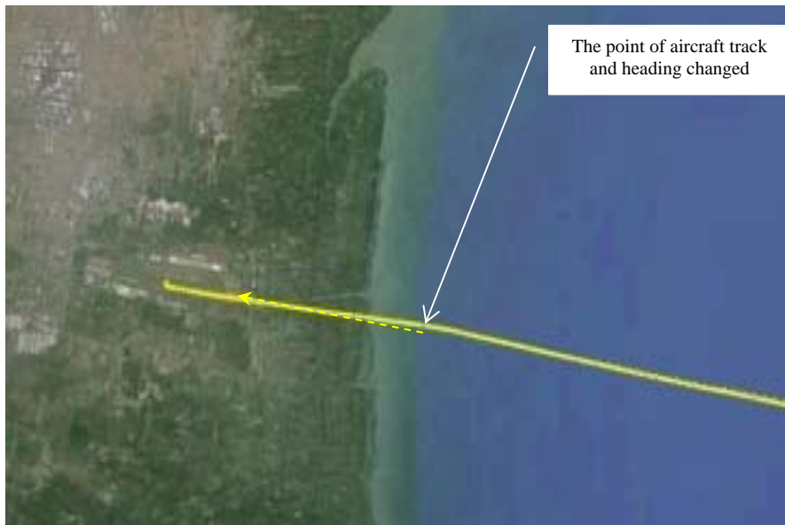
Figure 10: Shows the aircraft heading changed from 283° to 277° at approximate 500 feet
