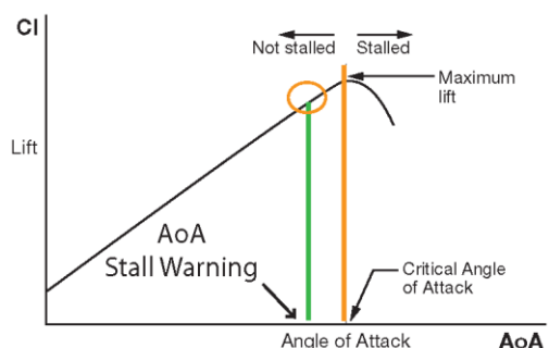
Figure 2 In ALTERNATE and DIRECT LAW, the aural Stall Warning is set at a value lower than AoA STALL.
