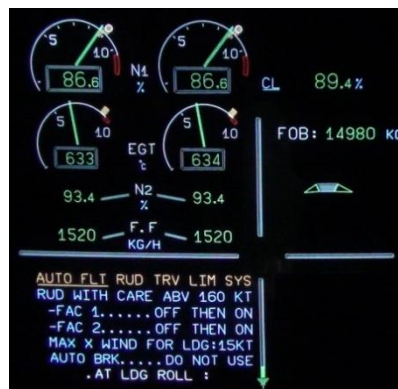
Figure 34: The ECAM messages after RTLTLU 1 and 2 fault
