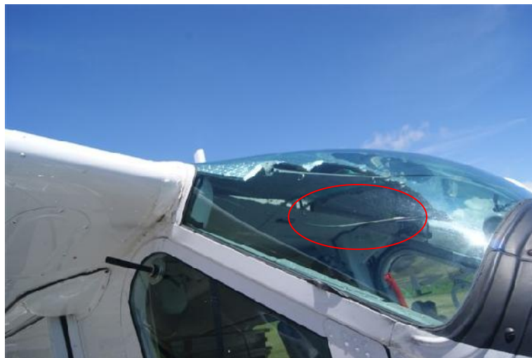
Figure 5: Windshield crack (red circle)
