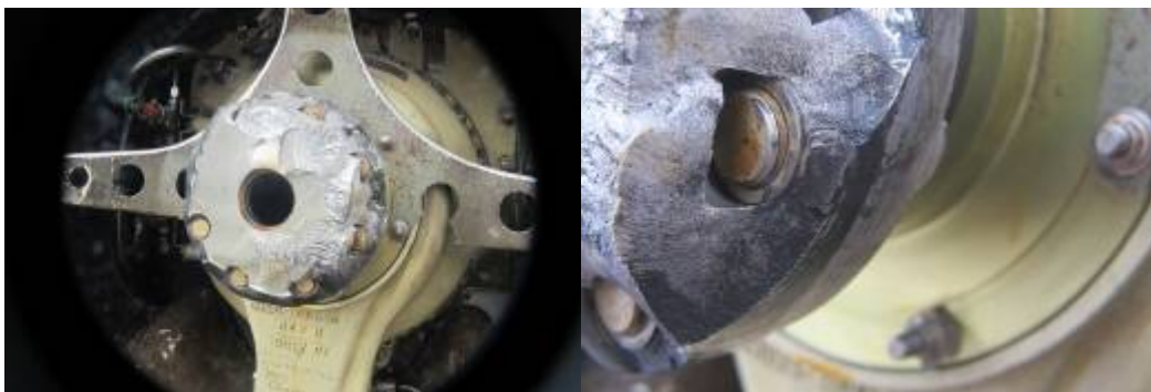
Figure 9: Remaining left propeller hub half attached at the propeller flange
