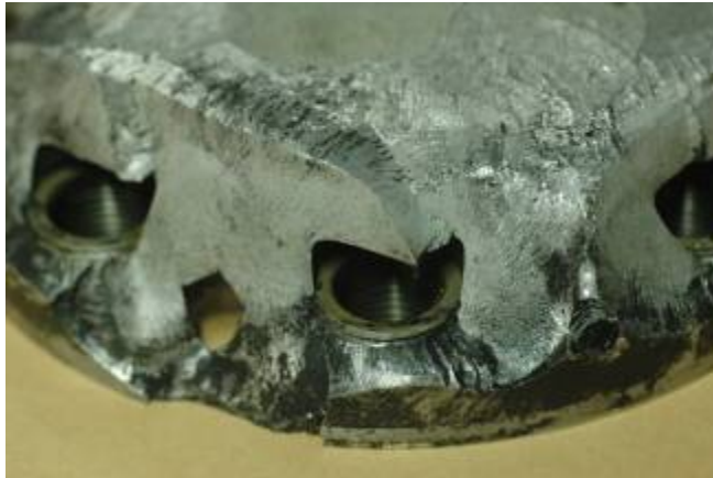
Figure 11: Fatigue cracks: darker surface shows earlier crack development while the lighter surface shows cracks developed somewhat later
