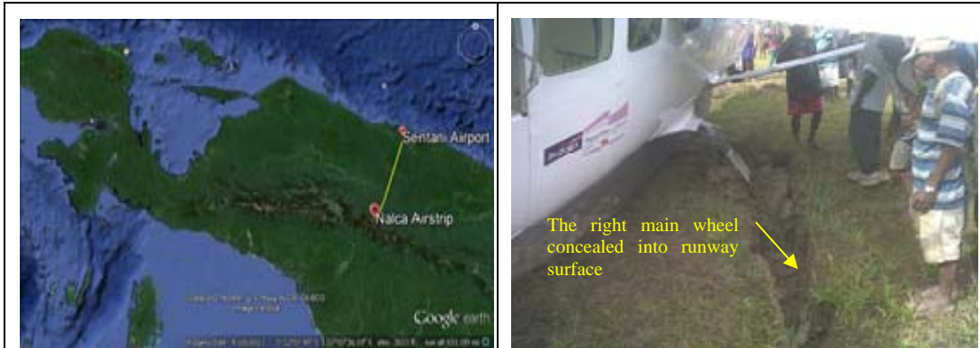
Figure 2: Shows the flight track and the right wheel concealed on the runway
