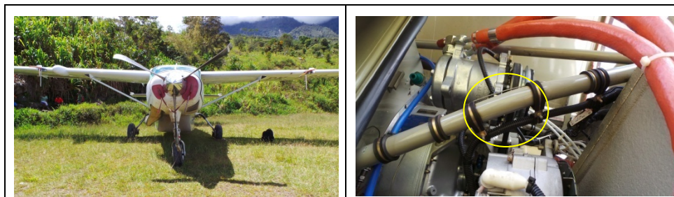
Figure 3: Shows the aircraft and the bend of engine mount in the circle
