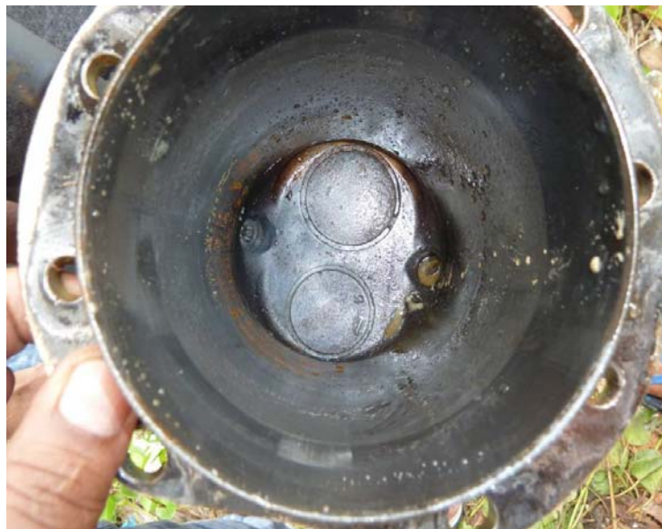
Figure 4: The damage found on the exhaust valve
