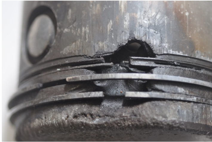
Figure 8: Burned and punctured area
