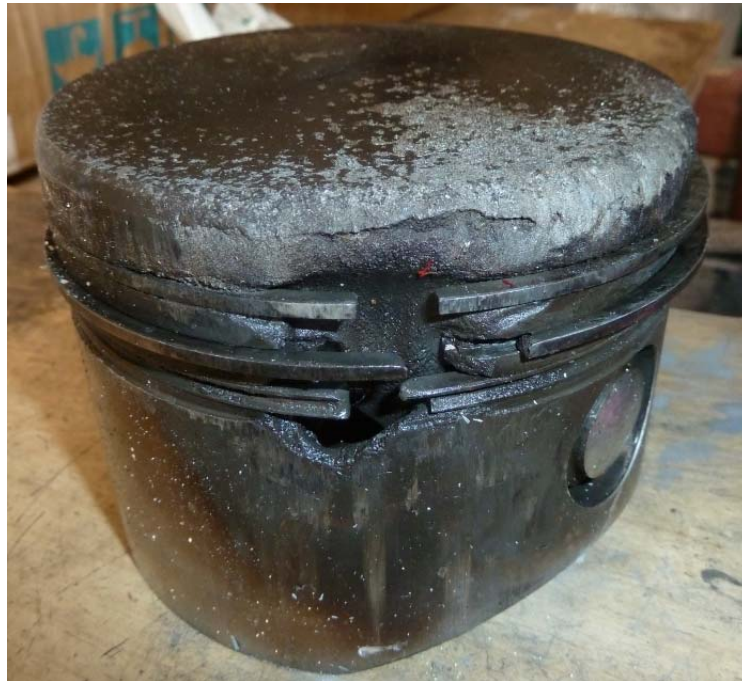
Figure 3: One of the melted and scratched pistons
