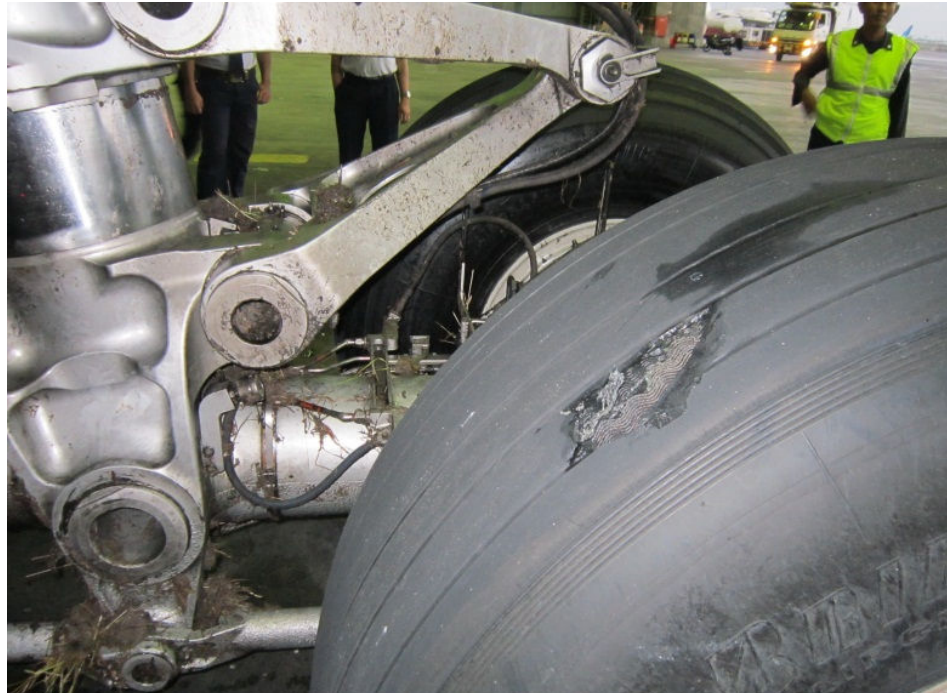
Figure 4: One of the tires torn and cut
