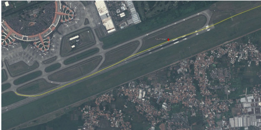
Figure 1: The flight trajectory and touchdown point revealed from the FDR and superimposed to Google Earth.
