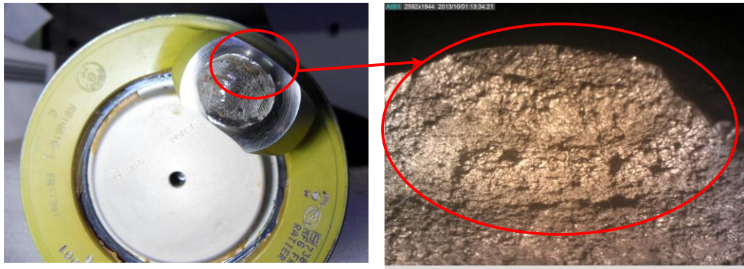
Figure 20: Crack initiation found on the trunnion pin of blade number 5
