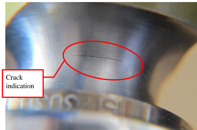
Figure 21: Crack indication on the trunnion pin of propeller blade number 2
