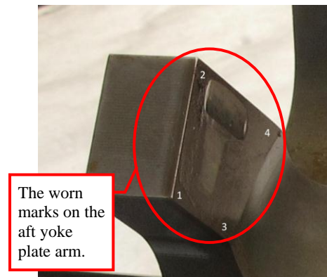
Figure 23: The worn mark on the one of the aft yoke plates
