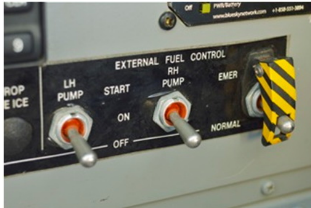
Figure 5: Auxiliary fuel control
