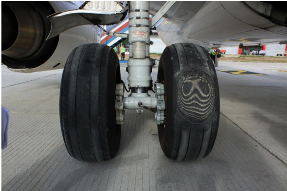
Figure 8: Spot and reverted rubber on the main wheel number 2
