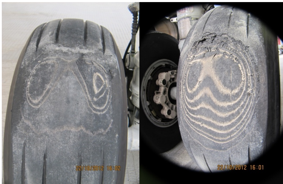
Figure 3: The tire damage found at inner side of both main wheels
