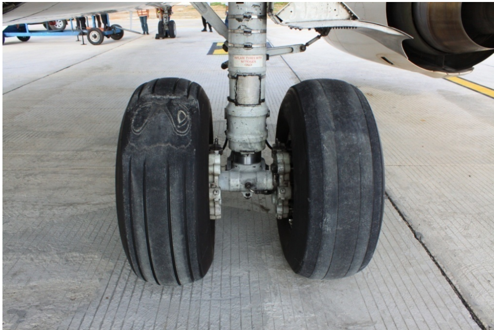
Figure 9: Spot and reverted rubber on the main wheel number 3
