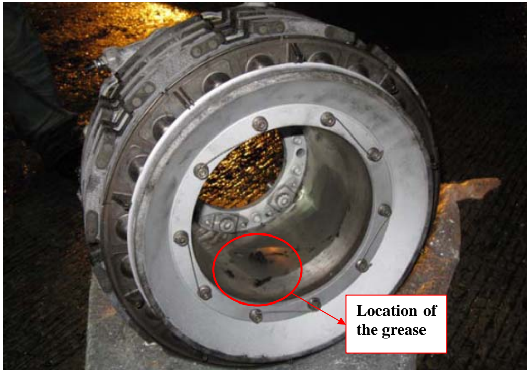
Figure 3: Residual grease on the brake number 2
