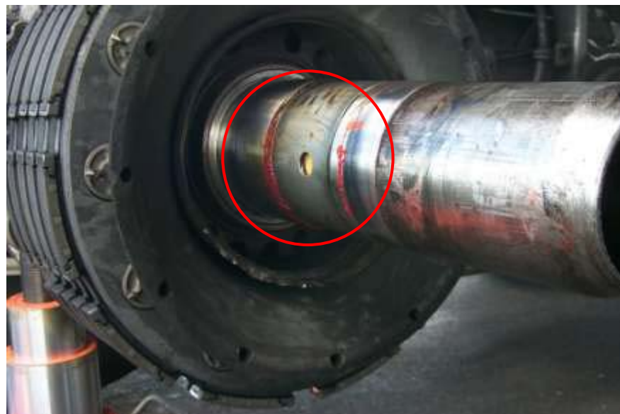
Figure 4: Hole that may allow excess grease to migrate to hot brake area
