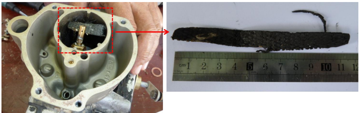
Figure 7: The rubber in the carburetor
