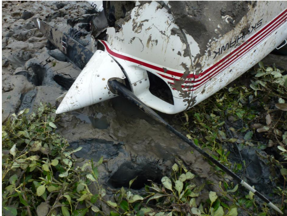
Figure 5: The propeller condition
