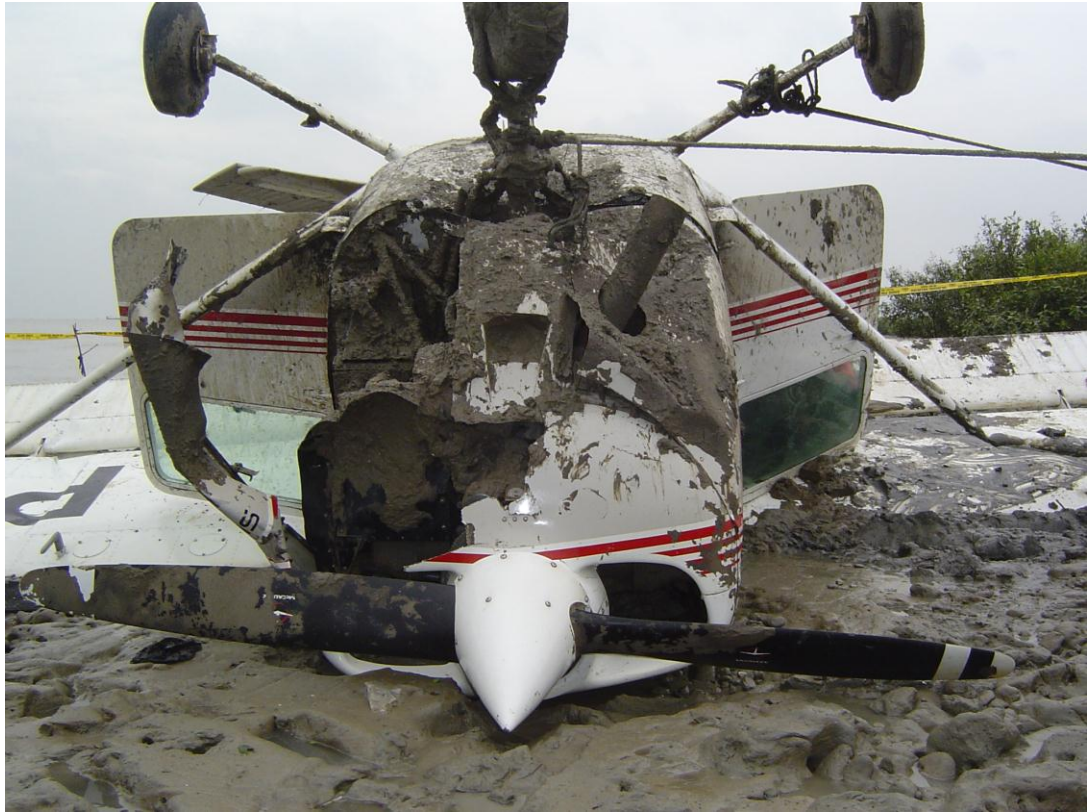
Figure 3: Broken on the engine cowling
