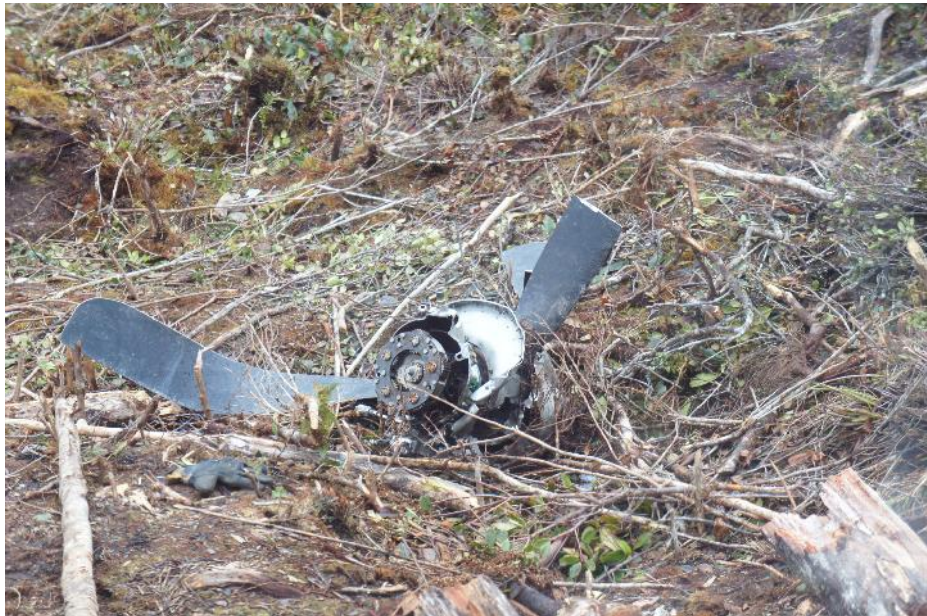
Figure 15: The detached propeller with two blades bent rearward (one blade cut for recovery)
