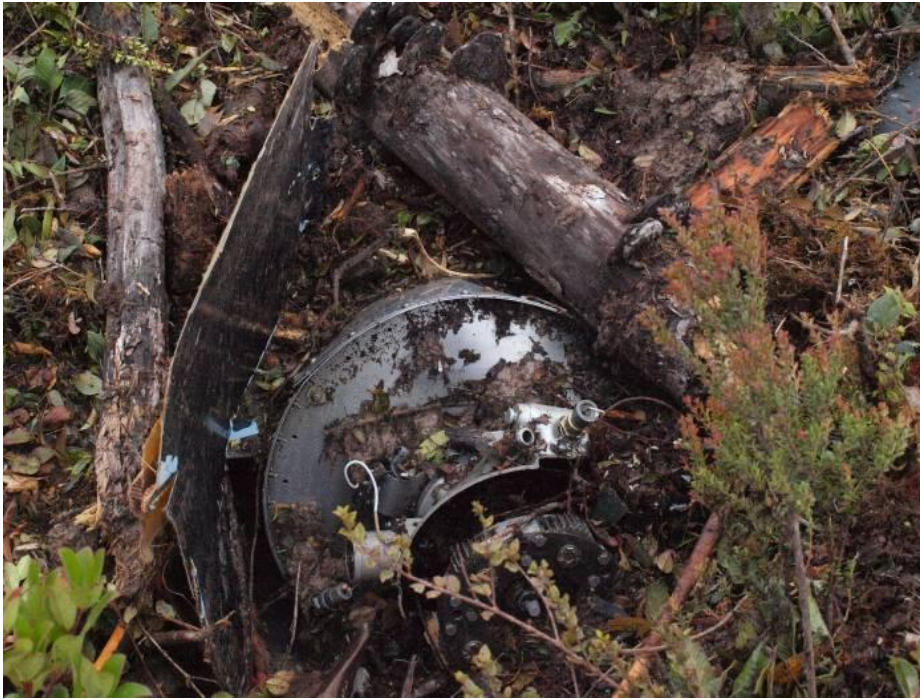
Figure 12: The Reduction Gearbox & Propeller detached from the engine
