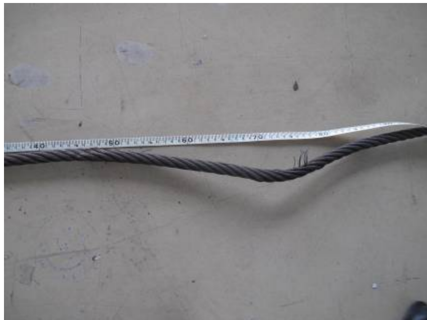
Figure 4: Damage on the sling cable
