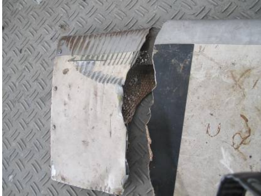
Figure 3: Tail rotor blade tip showing evidence of contact with cable
